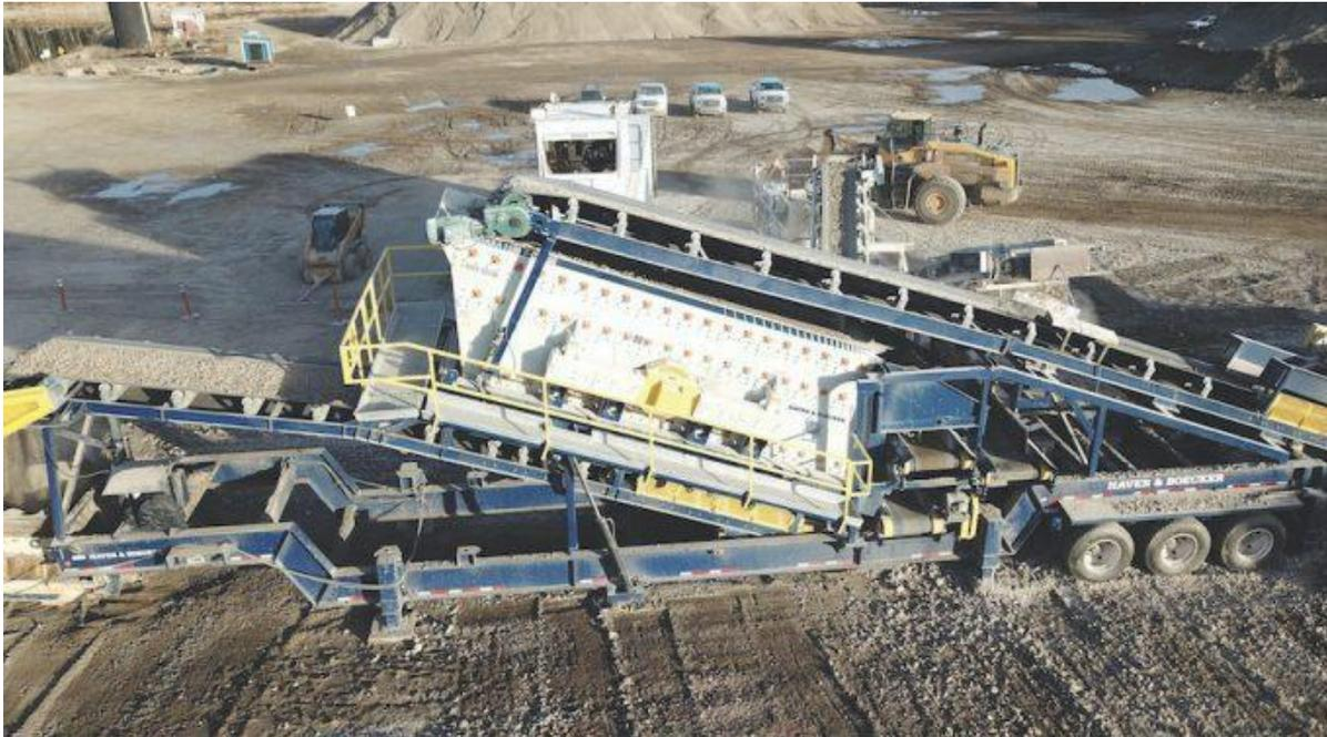
Haver & Boecker Niagara, Haver & Boecker's new mineral processing brand, offers the Niagara F-Class portable plant. The circular motion inclined vibrating screen allows operations to increase production by 25 per cent while making screen media change-outs easier on an inclined vibrating screen.
