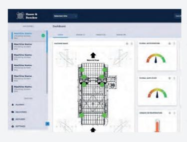
The main tab of the monitored vibrating screen contains its most valuable information, allowing the user to have a full overview of the equipment at that moment. Thenext few tabs will be specific for each of the body and bearing sensors. The graphic displays of the main parameters allow users to easily identify the equipment's operating condition and check if important parameters are within the established limits. Moreover, thresholds will be provided to guide the analyst.
